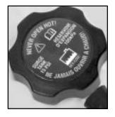
1. Park the vehicle on a level surface. You can remove the coolant surge tank pressure cap when the cooling system, including the coolant surge tank pressure cap and upper radiator hose, is no longer hot.
